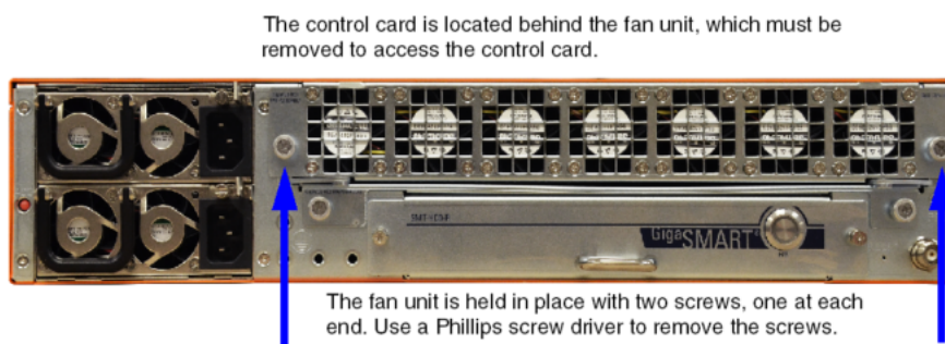
Figure 1 Replacing a Control Card
